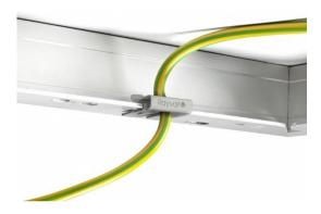
Alternatively, it is possible to connect the main ground wire to the HeliosLite Single or Double panel fastening brackets using standard grounding lugs. In this case, it is important to insure that the main grounding wire remain continuous if one of the grounding lug is temporally disconnected during a maintenance operation on the plant.
